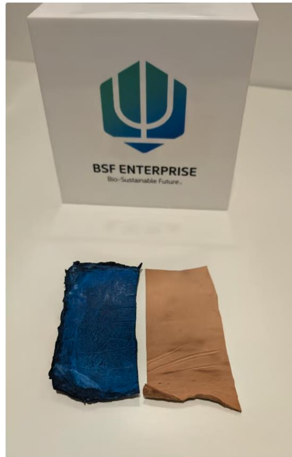
Figure 5: Lab-grown leather (left) produced via a partnership between BSF and the University of Northampton (Fashion United UK).
